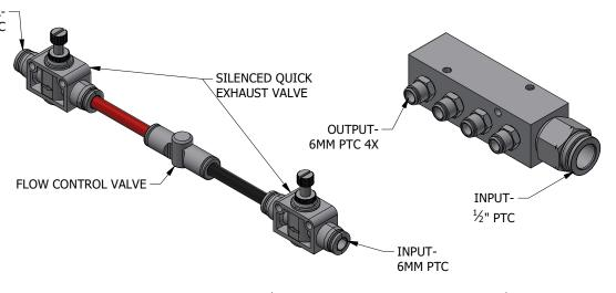
FLOW/EXHAUST VALVE ASSEMBLY
