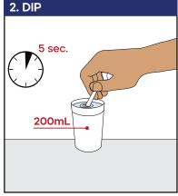
Gently dip ozone test strip into a **200mL** room temperature water sample for **5 seconds** with a constant, gentle back and forth motion (10 half strokes).
