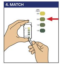
Match to the color chart at 30 seconds. Tersano SAO concentration is approved at **0.3ppm**\*. A colour match at 0.5ppm exceeds the approved sanitation range testing.
