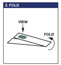
For best color matching, fold the white plastic handle of the test strip under the aperture so that it produces a white viewing background.
