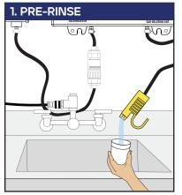
Ensure that testing container has been pre-rinsed with SAO solution for each dip test.
